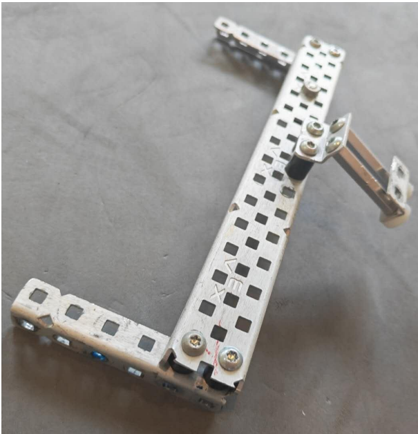
Close up of the new roller to help push the balls out of the middle scoring mechanism.
